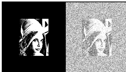
Figure 12: Grayscale Lena converted to pure black and white by thresholding (left), and the BBC codeword generated when that is used as the target image (right).
